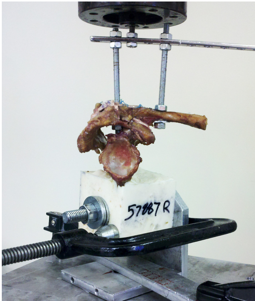
Figure 3. Biomechanical testing setup showing the potted scapula secured to loading platform of the MTS machine. After preconditioning, a tensile load on the clavicle in the superior direction was imparted until failure of the AC joint.
